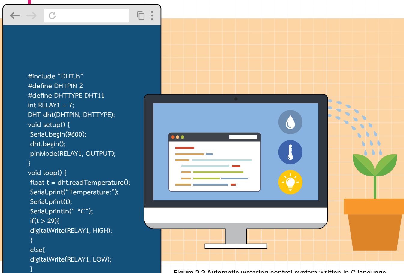
Figure 2.2 Automatic watering control system written in C language.
